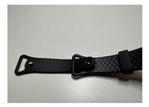
Slide the narrow end of the Strap Extender through the Nymi Band loop. Make sure the mushroom metal peg on the extender is pointing upwards.
