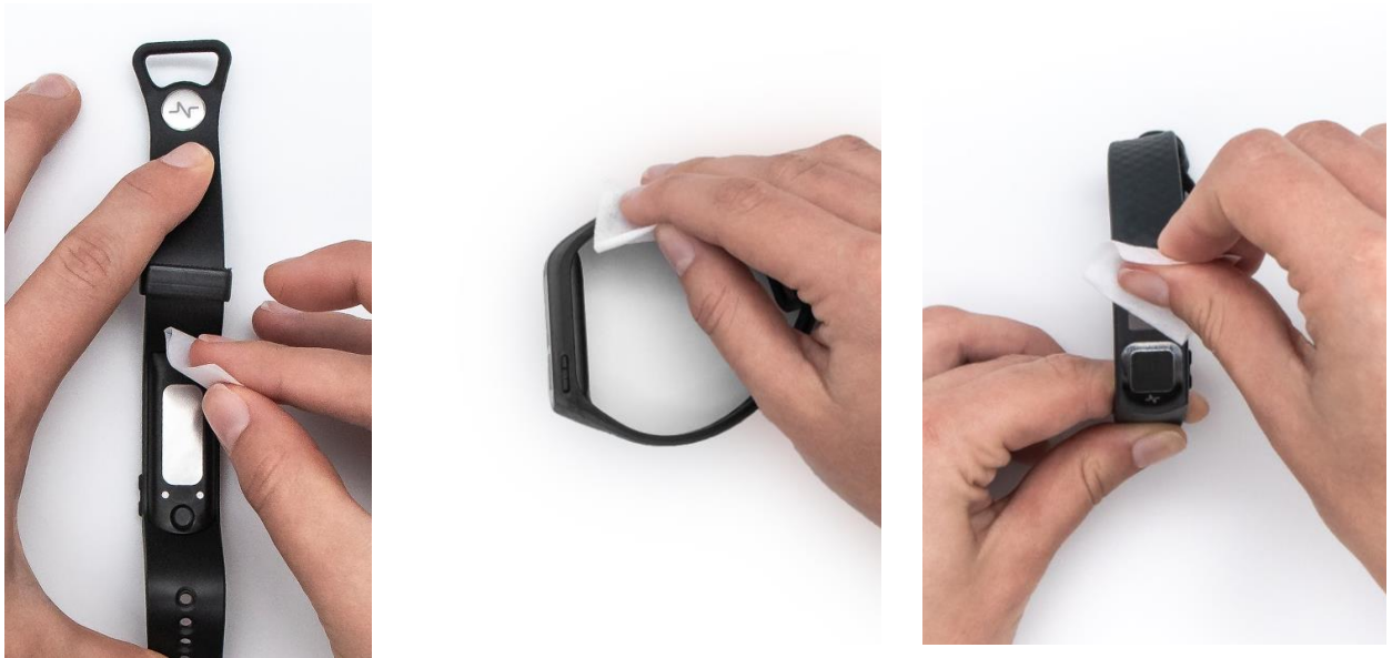
Figure 1: Wiping the Nymi Band's body and straps with an isopropanol wipe
