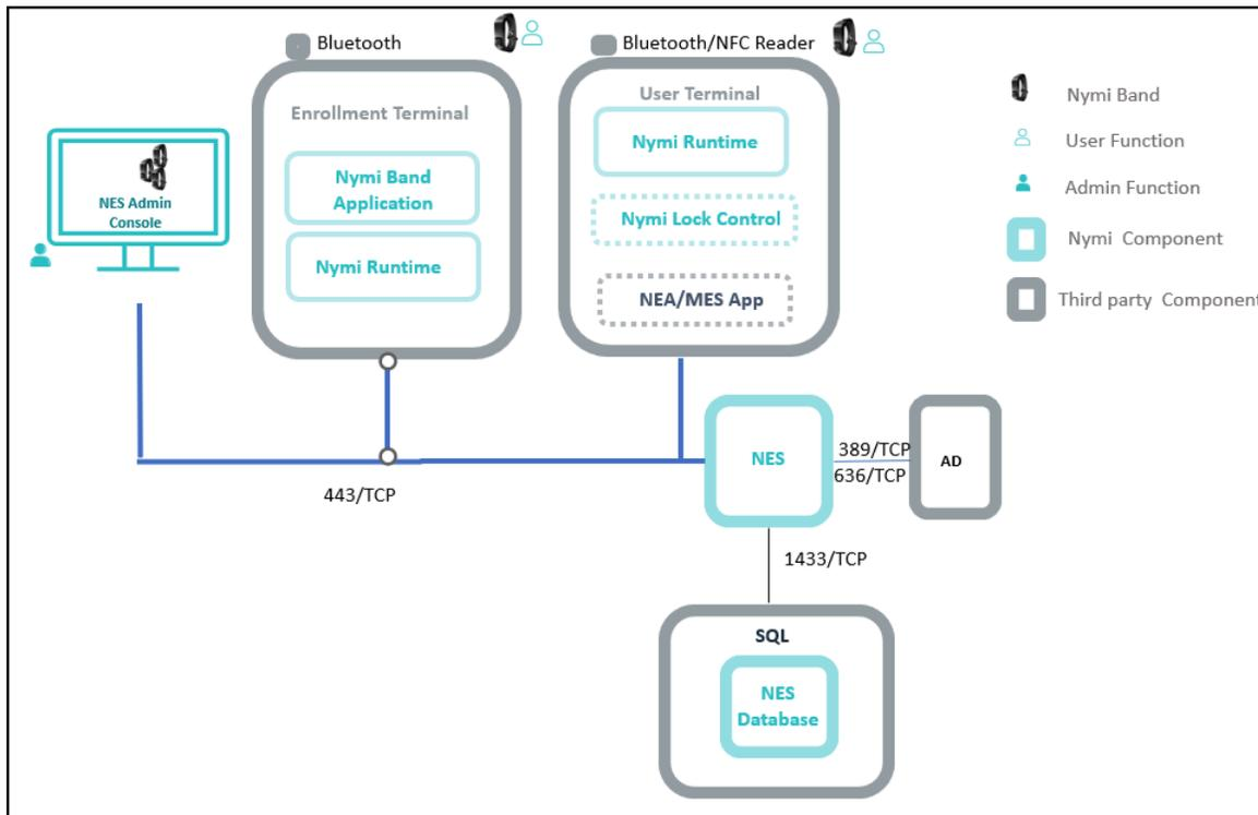
**Figure 1: Connected Worker Platform components and connection ports**
