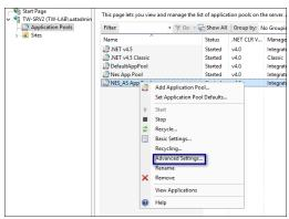
Figure 18: Advanced Settings for Application Pool
