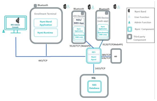
Figure 1: CWP components and firewall connection ports
