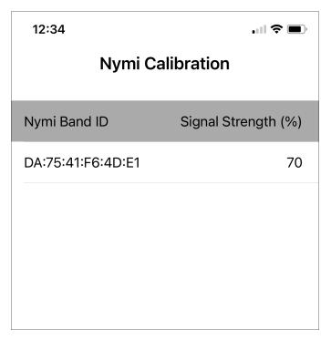
**5.** Place a sticker over the location on the iOS device that has the highest signal strength value.
