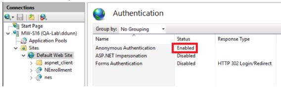
Figure 17: Authentication pane with Anonymous Authentication enabled
