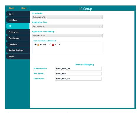
Figure 11: IIS Setup page in the NES Setup wizard
