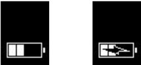
**Battery charge indication when off charger (left) and on charger (right)**
