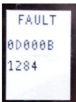
Figure 7: Nymi Band Screen with a Fault Condition
