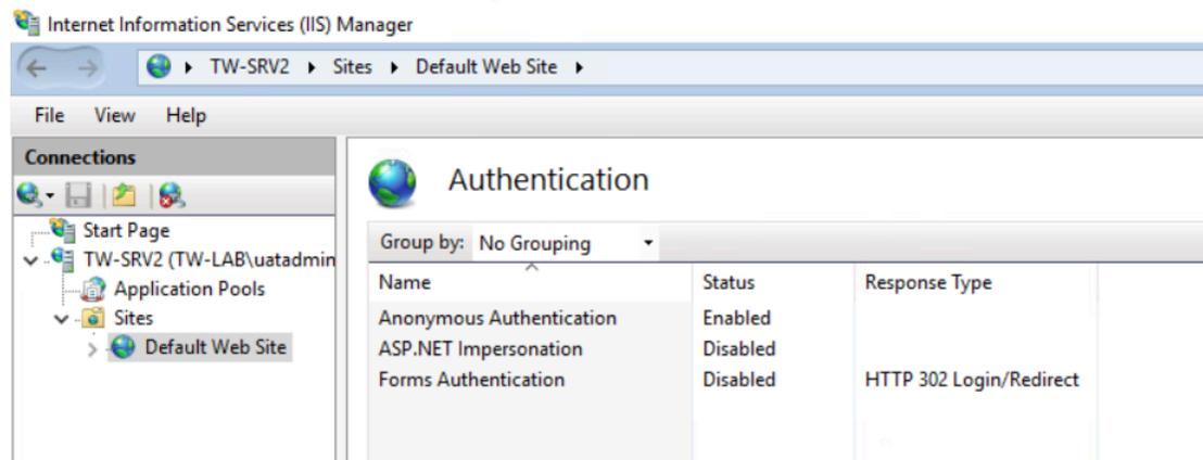
Figure 16: Authentication pane with Anonymous Authentication enabled
