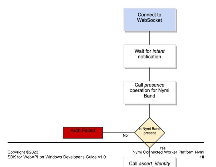
In both authentication examples, the first step is to wait for an intent notification. The intent operation tells the application that a user has placed their Nymi Band on an NFC reader that is connected to the workstation. The intent operation returns a device ID, which is the standard identifier of a Nymi Band in the CWP solution.
