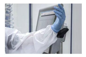
Through the Nymi Band's On-Body Detection feature, workers can access physical areas and authenticate to computer systems without touching any equipment. This reduces overall user movement and contact with communal surfaces where transfer of contaminants are more likely to occur. An employee wears and activates their Nymi Band at the start of their shift, before gowning.
